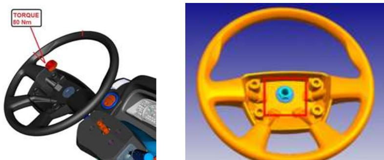
For 18 MY, W719428 S439 numbered bolt connecting the steering wheel to the column will be tightened to 80 N.m.
