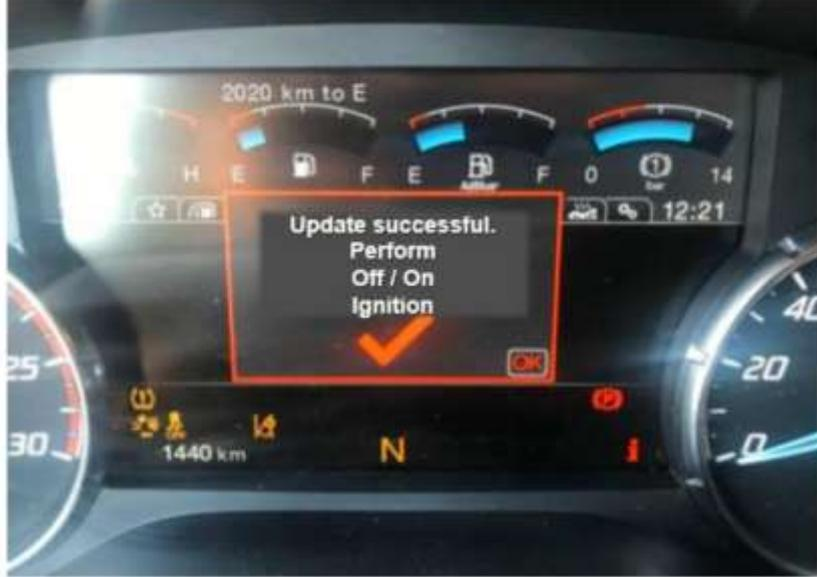
The above update successful message will appear on the display panel for 5-15 seconds and will disappear automatically. Do not turn off the ignition during this time and wait for the message to disappear. After a certain period of time after the message disappears, the contact can be turned off and on.
