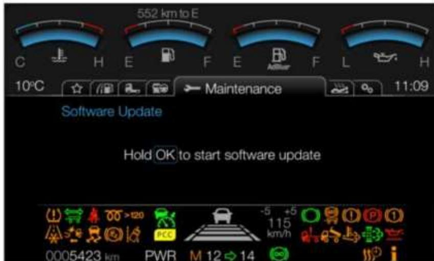
6. In order to start the software update, the vehicle is stationary, the parking brake is applied, the ignition is in the 2 position and the engine is not running, press the "OK" key for 5 seconds and release the OK button when the progress bar is full.
