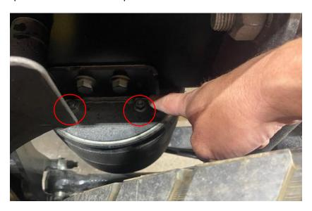
Remove bottom bracket bolt and then remove rear C4AS suspension air bellow Install new rear C4AS suspension air bellow (DC46 5580 DB)
