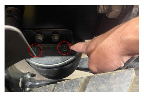
Remove bottom bracket bolt and then remove front C4AS suspension air bellow Install new front C4AS suspension air bellow (DC46 5580 CB)
