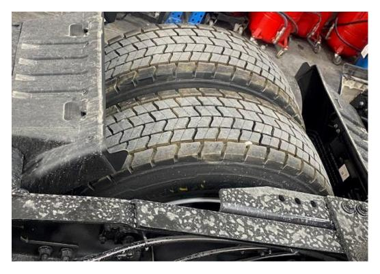
Put into higher positon for air bellows with ECAS and then put calibration block between right-left chassis and rear axle.
