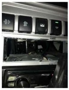
• The connections of the new version DTCO 4.1 tachograph are also compatible with the old version tachograph connectors that have been removed. The connectors and antenna wirings of DTCO 4.0 should be plugged to the DTCO 4.1 version Smart Tachograph.
