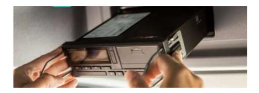
• The electrical wiring connections and antenna wiring connectors should be unplugged from the DTCO 4.0 tachograph.
