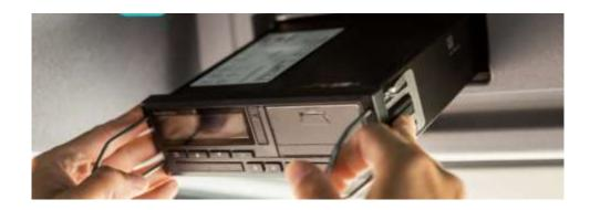
• The electrical wiring connections and antenna wiring connectors should be unplugged from the DTCO 4.0 tachograph.
