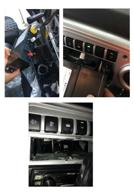
• The connections of the new version DTCO 4.1 tachograph are also compatible with the old version tachograph connectors that have been removed. The connectors and antenna wirings of DTCO 4.0 should be plugged to the DTCO 4.1 version Smart Tachograph.
