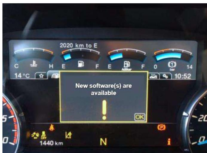
3. This message will be displayed as a reminder each time the ignition is switched on if the software update process has not been started in the vehicle.
