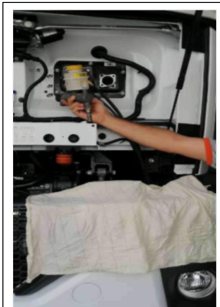
Image 1 - The areas on the vehicle where oil can spill should be covered with a cloth
