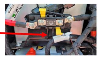
The plastic push-pin should be mounted to the bolt via the sponge.
