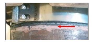
Tighten the V-clamp (GC46-9N435- AA) in Figure F to 19Nm.
