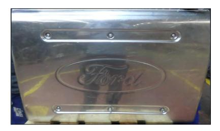
18- Tighten 9 bolts (W505541 S437) on the upper heat shield of the muffler (**GC46-5K277-BA**) to **25+/-4 Nm** using a 6" allen wrench.
