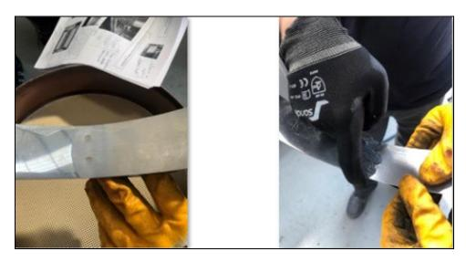
8- Engage the clamps to the DPF with the V-Clamp first, then the stopper clamp and finally the Tape Clamp as shown in **Figure C** respectively.
