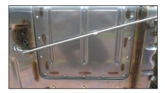
16- Install 2 suspension brackets (**GC46-5A277-AA**) where the heat shield with Ford logo is installed and 4 bolts (**W505541 S437**) on it using a 6" allen wrench and tighten the bolts to **25+/-4 Nm**
