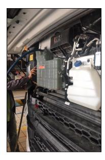
11-Run the engine above the idling speed and wait until the thermostat turns on. You may understand that the thermostat is turned on from the vibration on the upper hose of the radiator or from the water flow inside the expansion tank. Run the vehicle for 10 more minutes after the start of the flow to ensure that the air inside the system is discharged. Check for leaks in the hoses. Switch the internal ventilation to the hot setting, and check if hot air is received.
