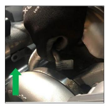
3- If you pull the pipe upwards, if there is no dislodgement, make sure that it is fit well by pushing it in the right direction.
