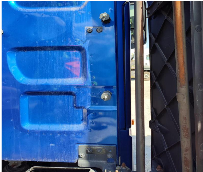
Figure 3: Retightening the bolts
