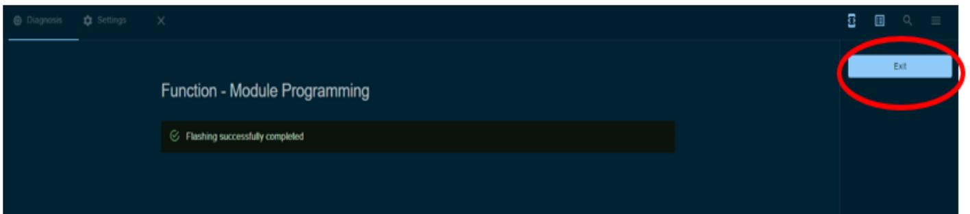
After module programming process has been completed, please check CGW parameters whether correct or not. If not, please write configuration parameters via FODiT.
