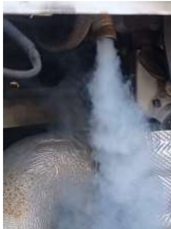
Image 1 - White smoke coming out of the heater exhaust.
