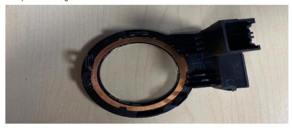
• Then, the PC46-19H447-A\* (Adapter Part) with the tabs on it and the part numberes JC46-021C04-A\* (Copper Ring) and 8A6T-15607-A\* (Pats Module) which have been assembled to each other are installed so that the tab slots are facing each other.
