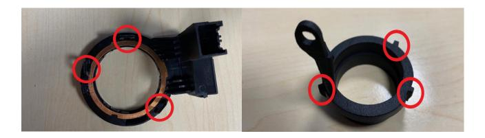
• Finally, the second copper ring with part number JC46-021C04-A\* (Copper Ring) is adhered to the other side of part number 8A6T-15607-A\* (Pats Module). Photos showing the process are shared below.
