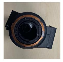
After these processes are completed, 8A6T-15607-A\* (Pats Module) will be combined with the part number HC46-3K772-A\* (Housing). Although the HC46-3K772-A\* (Housing) is a common part in Yanfeng and Nidec modules, if the HC46-3K772-A\* (Housing) is damaged, the HC46-3K772-A\* (Housing) should also be replaced.
