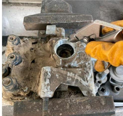
**Place new silencer (JC46-2D014-A\*) and hand tighten as indicated direction.**
