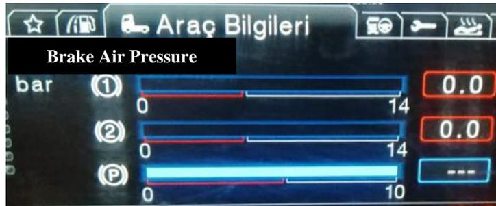
**Check if E-APU exhaust port drains air continuously under 5.5 bar or not**
