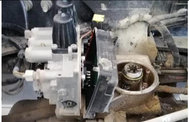
Replace all 3 pressure sensors and assemble the E-APU by following the above steps in reverse order.
