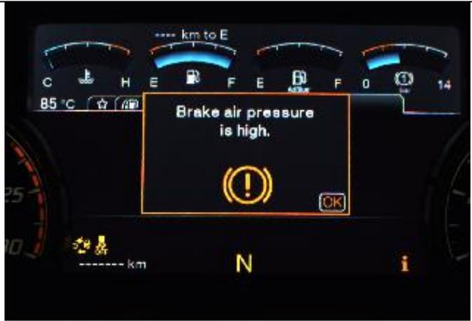
2) If there is a "**Brake air pressure low**" error, then brake pedal is pressed repeatedly until the pressure values of all circuits decrease below 5.5 bar.
