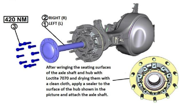
7. Tighten 10 x M24 axle cover bolts (DC46-4N100-AA) to 420 $\pm$ 20 Nm.
