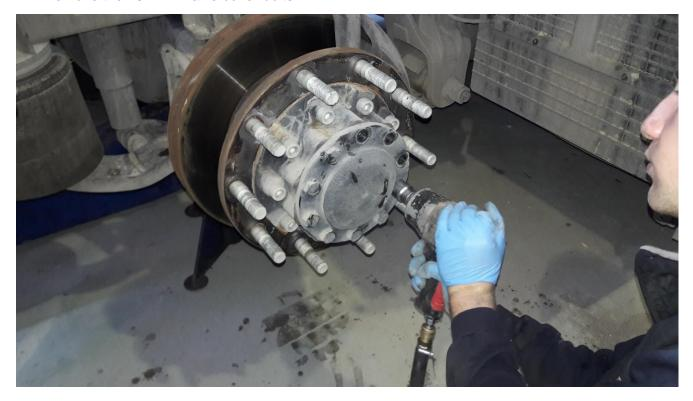
**3.** Carefully remove the axle cover using a screwdriver because damage on the parts may lead to claims in the future.
