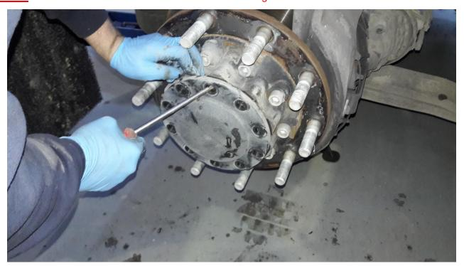
**4.** Remove the old level hub nut and old level washer using SST H050205-LA (special tool) which can be seen in right bottom of the page. Old level hub nut: HC46-1A124-AA (Right Wheel) / HC46-1A125-AA (Left Wheel) / Old level washer: HC46-1124-BA
