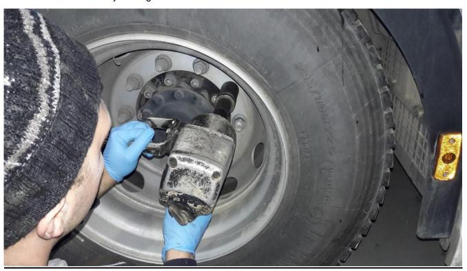
2. Remove the 10 x M24 axle cover bolts.
