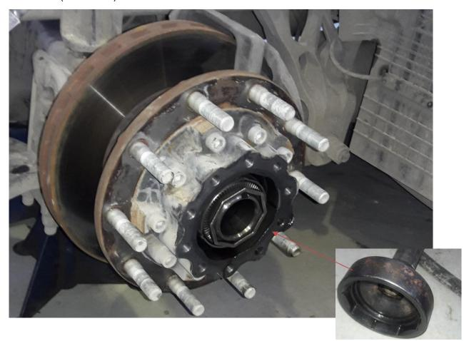
5. Install the new level washer (HC46-1124-BB) with the pin part inside the axle shaft groove. After the washer, torque the new level nut to 950±50 Nm using appropriate equipment. After the nut is torqued, drive the nut where it coincides with the axle shaft housing as shown below.
