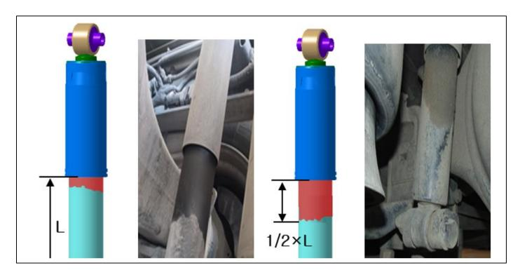
The situations in which shock absorber does not need to be changed are shown.
