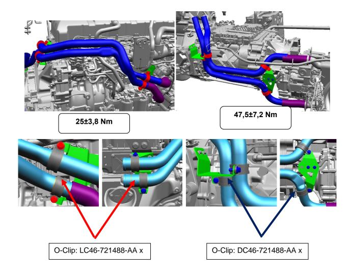
Insert hoses to metal pipes and position as per the aligning lines. Then, tighten the clamps and complete the operation.
