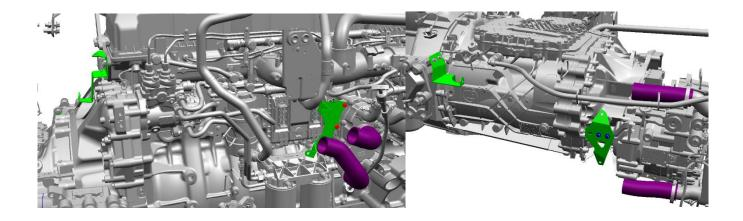
Place new metal pipes to their positions and position the O-clips between the markings. Then, tighten the bolts to the specified torque values.
