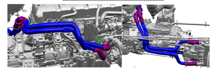
Remove the connection bolts of metal pipe brackets.
