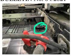
When the vehicle is in-service, BMOS connector must be removed and installed, and if the warning lamp is
