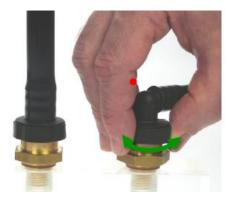
2- Press on the part shown below and pull the hose in the direction of arrow. (The point to be pressed on some parts is marked with a white paint)
