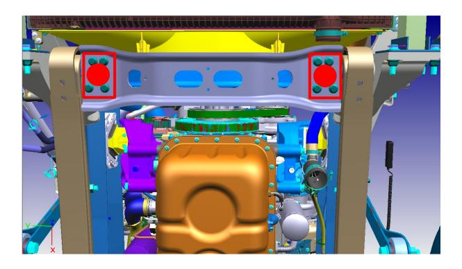
**3)** Please loosen 4 x M20 U-bolts of the suspension spring and slightly lift the vehicle with jack for providing make clearance to put caster shim.
