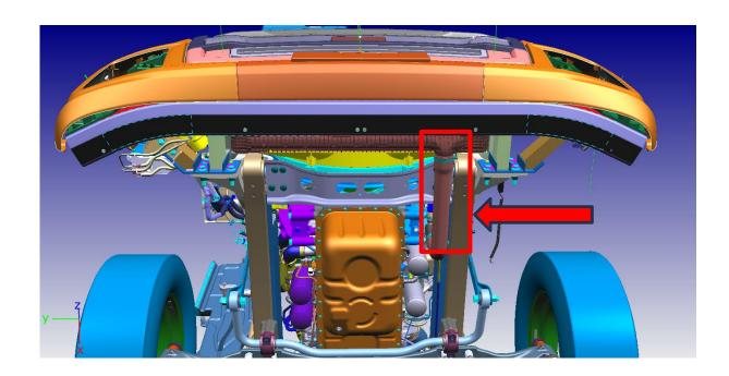
2) Place jacks with sufficient capacity under the indicated location below the chassis make sure jack sit properly and then lift the vehicle slightly.
