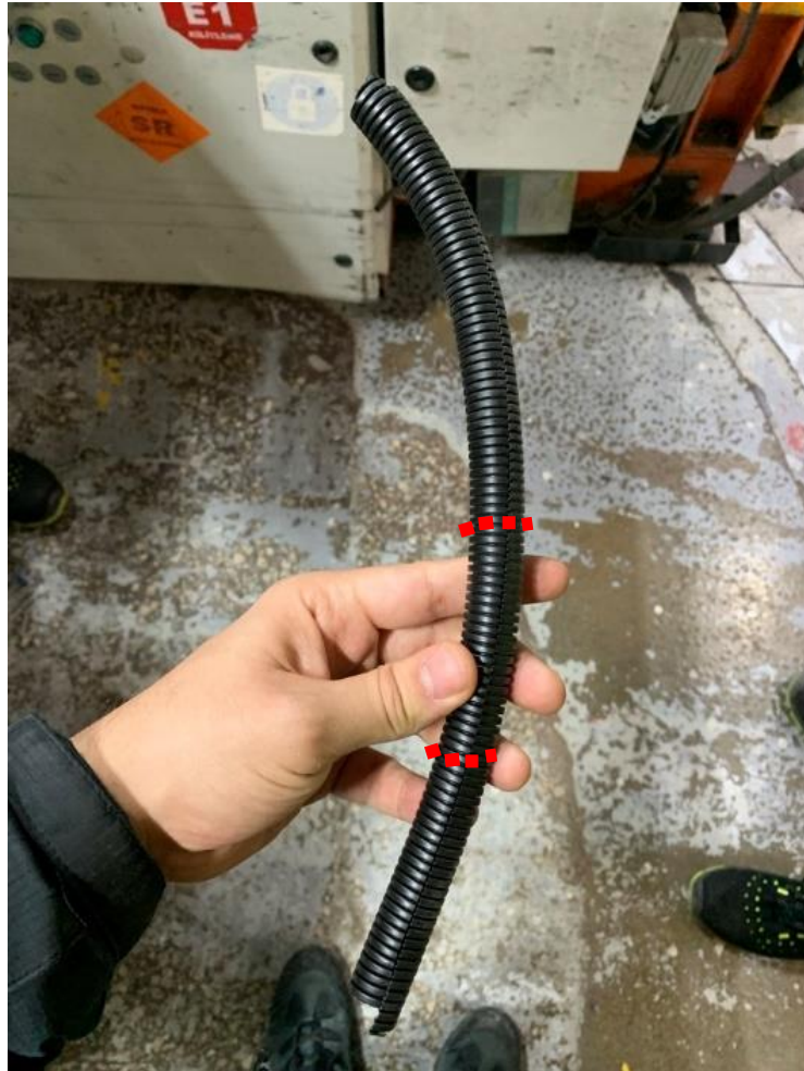
Figure 15 – GAF – 4C46-2254-BA – should be 10 cm long
