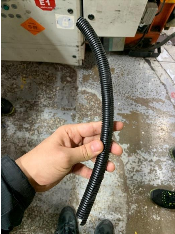
Figure 10 – GAF Part – 4C46-2254-BA – needs to be 15 cm long
