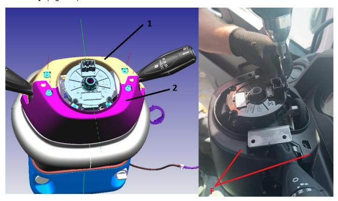
7. Remove the two connectors and three smounting bolts of the clock spring. Remove the clock spring and SAS sensor together without separating them. (Figure G)
