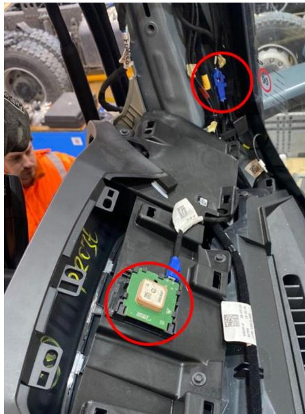
The new GNSS antenna wiring to be installed on the DTCO 4.1a tachograph should be routed along the A pillar and, with the help of a tool, brought to the headliner area. To allow the cable to pass through the marked area, first a guide air hose or another cable must be routed through the A pillar up to the beginning of the A-pillar. Then, the TC46-18812-BHA should be taped to the end of this air hose and pulled carefully through to the A-pillar opening without causing any damage.
