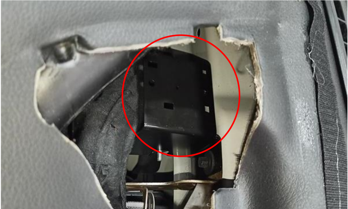
The GNSS antenna bracket is highlighted within the red circle in the image
