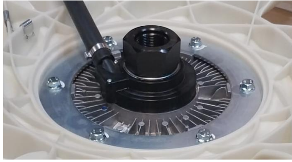
Figure 6 : Engine cooling fans have 6xM8x1.25 screws.
