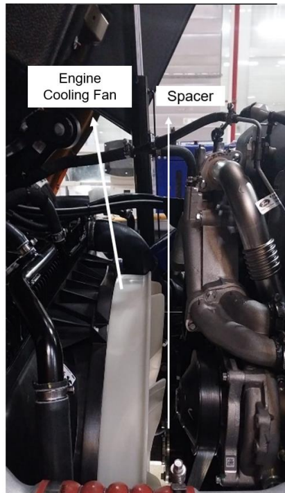
Figure 5 : Engine cooling fan and spacer parts after the cabin lift.
