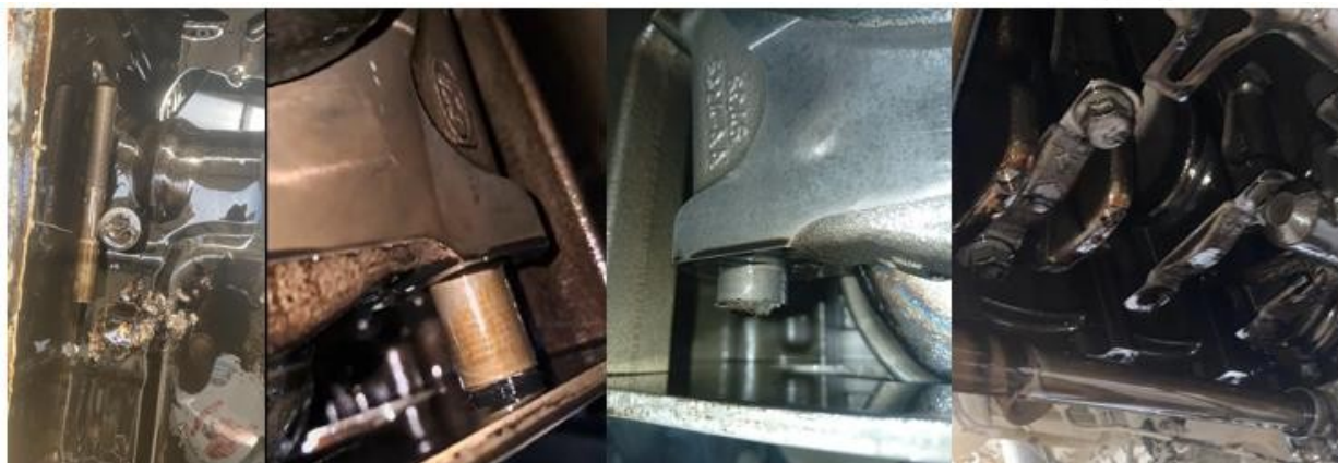
Damaged Main Bearing Cap Bolts
